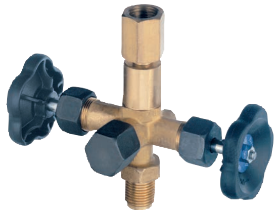
Shut-off valve with separately isolated test connection per DIN 16272, LH/RH union/male G 1/2, with test pivot M20 x 1.5, PN 400
